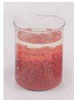
经Polymer加药调理反应后污泥形成胶羽凝结 After chemical disposal and reaction with polymer solution.
