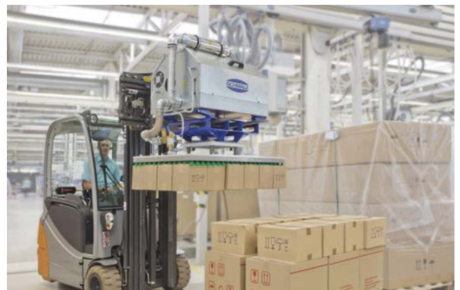
Vacuum layer gripping system SPZ on a forklift for picking cardboard boxes
