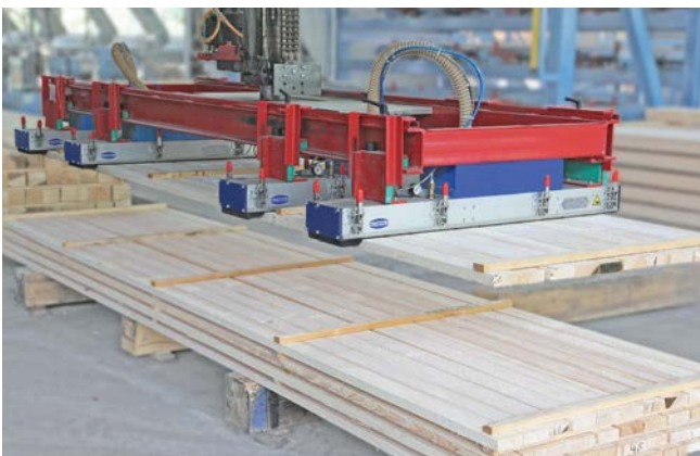
Vacuum area gripping system SBX for handling layers of wooden boards
