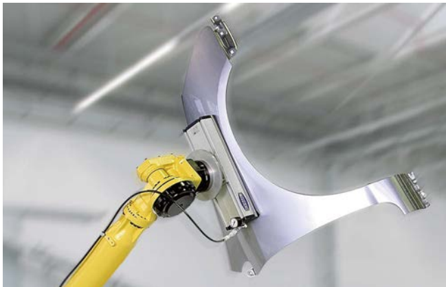
Vacuum area gripping system FXP being used to handle car body parts in the body shop
