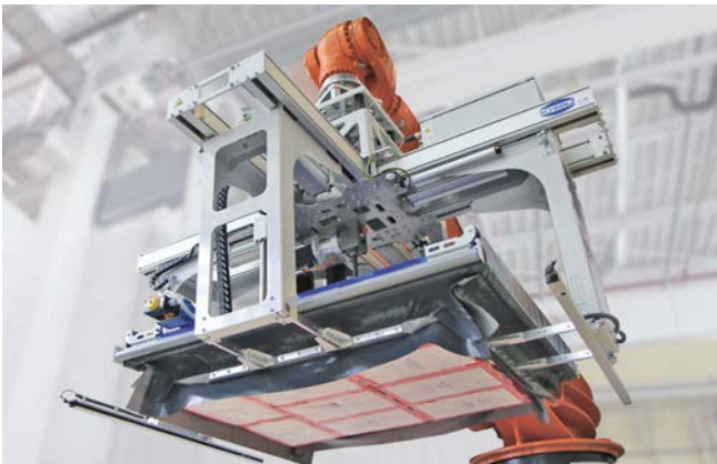
Vacuum layer gripping system SPZ-M-C being used to palletize beverage trays
