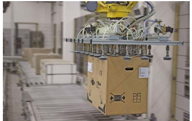
Vacuum suction spider SSP being used to pick boxes in a goods distribution center
