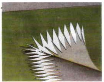
DOUBLE Z. it is executed on all conveyor belts with 2 or 3 plies; it ensures a high quality standard
