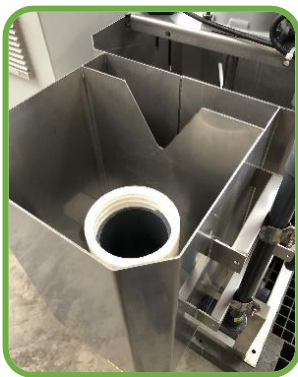
Laser cutting stainless steel SUS304 for Sludge water tank and Polymer mixing tank.
